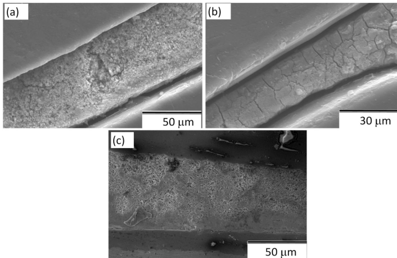
Fig. 1. Lower magnification SEM micrographs illustrating cross-sections of melt-spun Al-10Ni alloys with different amount Sc content; (a) base alloy (MS0), (b) 1 wt% Sc added alloy (MS1), (c) 2 wt% Sc added alloy (MS2)
