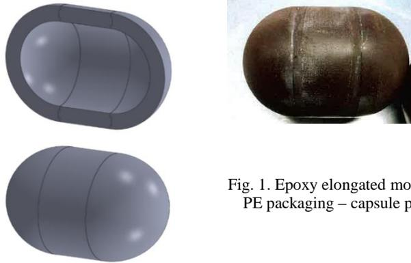
Fig. 1. Epoxy elongated module for PE packaging – capsule profile
