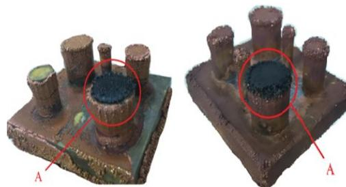
Fig. 10. Cortical EIs after processing in the EDM machine. A is the processing area
