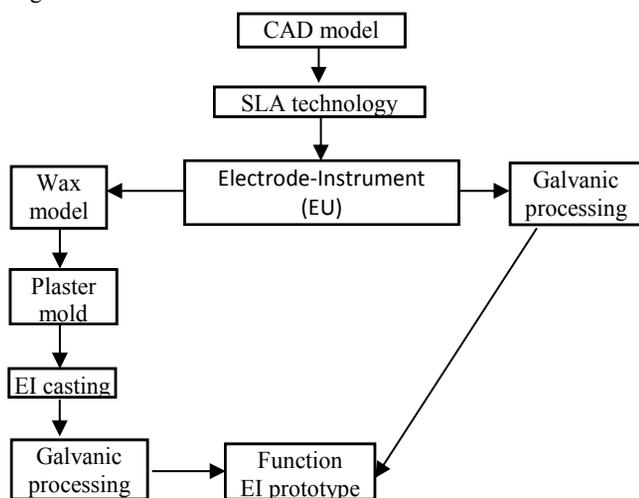
Fig. 1. The scheme of making a cortical EI by indirect methods with the use of rapid prototyping technology
