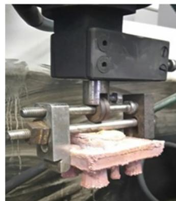
Fig. 9. EI fixed in the EDM machine.
