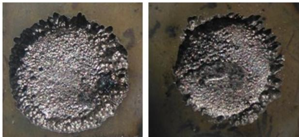
Fig. 11. The surface of the steel workpiece after EDMing with cortical EIs: a – imprint after treatment with cast EIs; b – imprint after treatment with EIs obtained through the RP technology
