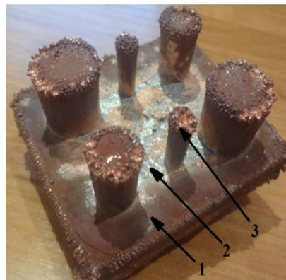
Fig. 7. A cortical EI obtained by casting after galvanic treatment: 1 – copper coating layer; 2 – uncovered areas; 3 – copper build-ups
