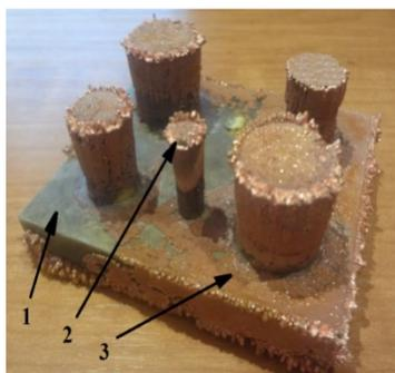
Fig. 8. Cortical EI: 1 – the primary conductive layer; 2 – copper build-ups; 3 – copper layer
