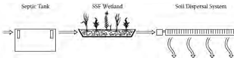
Fig. 13. Deep flow wetland and septic waste treatment; source: KADLEC and WALLACE [2009], modified
